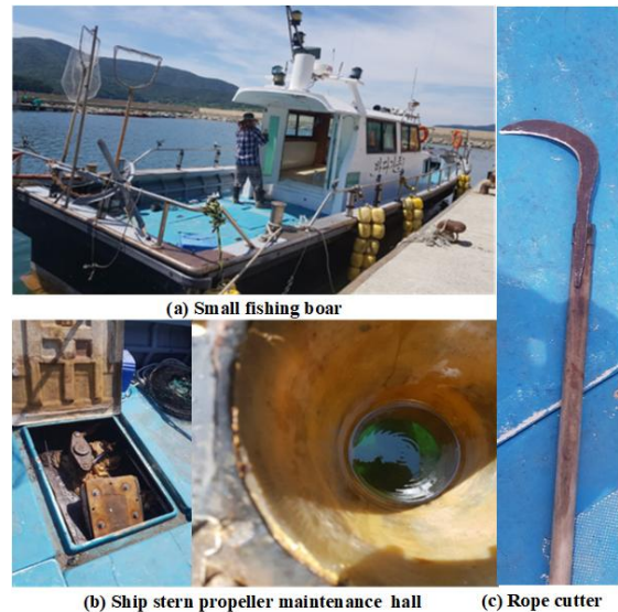
Fig. 2. Ship maintenance hole.
