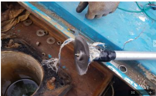
Fig. 4. Circular-top blade cutter failure.
