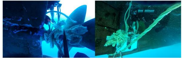
Fig. 1. Accident due to foreign substances wrapped in the propellant (Kpilbo, 2017).
