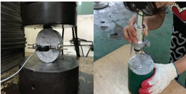
Fig. 1 Inducing crack to fly ash concrete specimens
