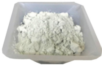
Figure 4. Precipitate produced after adding oxalic acid to lactic acid leached CAMP.
