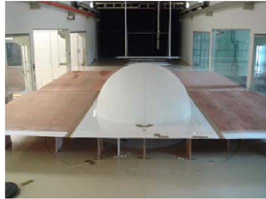
〈Fig. 4〉 Hemispherical pressure models in smooth flow wind tunnel<sup>1)</sup>
