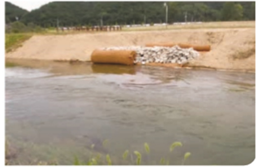
(b) Operation test of rolling mat
