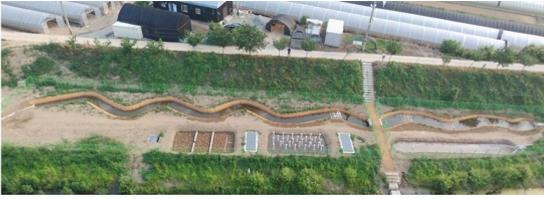
Fig. 3. The test bed of sheet flow channel in the Osan stream.
