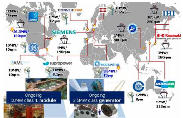
Fig. 1. Global trends of superconducting wind generators.
