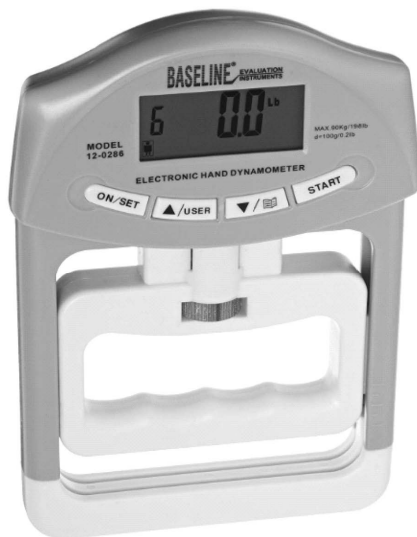
Fig. 2. Baseline digital smedley spring dynamometer.
