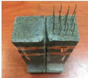
(e) UBH16 After Tests (Hooked Fibers)
