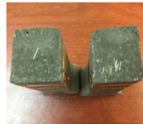
(f) UBT16 After Tests (All Twisted Fibers Broke)
