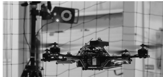
Fig. 1. A VICON camera and its reflective markers on the drone
