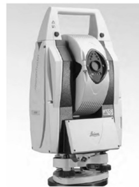
Fig. 2. A laser tracker system (Highly accurate point coordinate measurement system)
