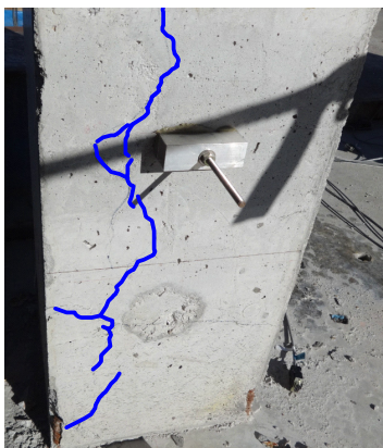
(e) visible damage on first story column base in as-built test frame
