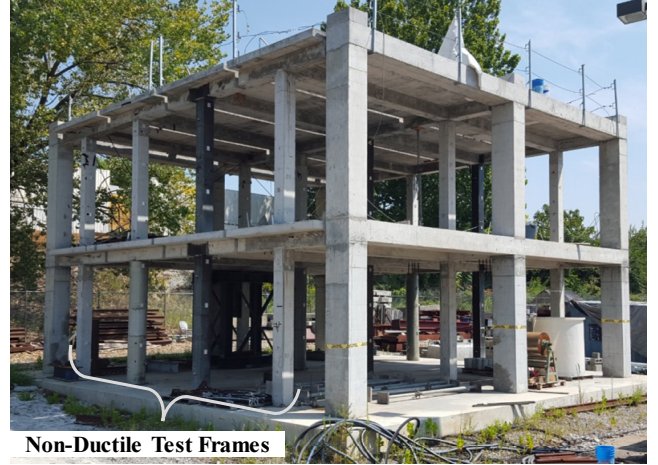
Fig. 3. Full-scale non-ductile RC test frames
