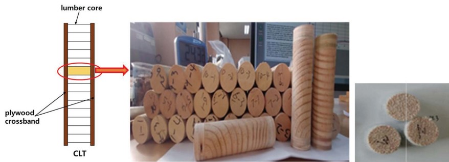
Fig. 1. Specimens for sound absorption rate measurement (left, CLT; light, polyester board).
