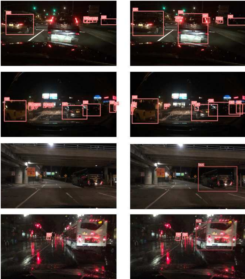
Fig. 6. The example results of the proposed method. Left images are results of YOLO algorithm trained using only Day class data, and right images are results of YOLO algorithm trained using Day class and synthesized Night class data. By the proposed method, YOLO can detect undetected objects such as a bus or cars under the night time.
