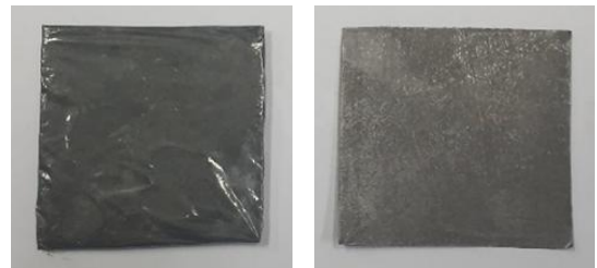
Fig. 1 Specimen with carbon ink (Left : Graphene Oxide@Graphite@Carbon Ink, Right : Carbon Nonwoven Fabric@Carbon Ink)
