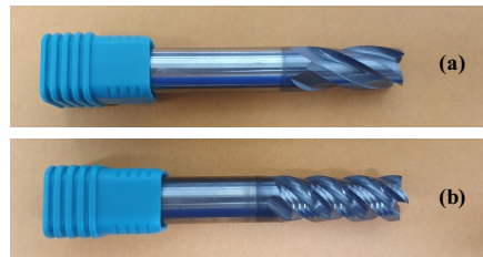
Fig. 2 Images of (a) general-purpose end-mill (TSE-4120M-TT5515), and (b) specially designed tool for titanium machining (SED-4120U-TT5515). Both have a diameter of 12 mm and from TaeguTec Ltd., Korea
