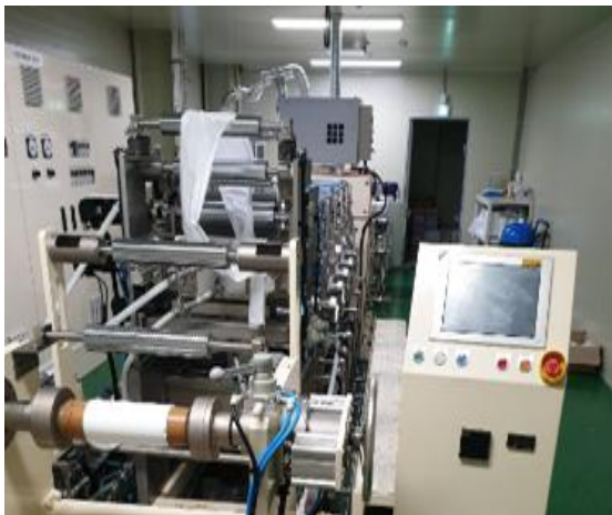
Fig. 5 Thermal stable separator coating machine
