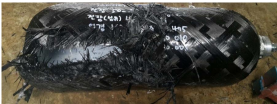
Fig. 9 Burst mode of liner for type 4 composite vessel
