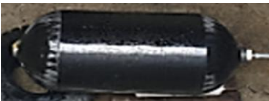
Fig. 10 leakage mode of type 4 composite pressure vessel
