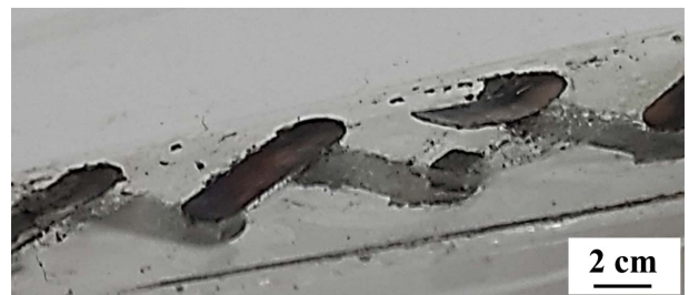
Fig. 7. Optical Image showing the joint failure between a Cu electrode and a thermoelectric leg at a strain of 0.2.
