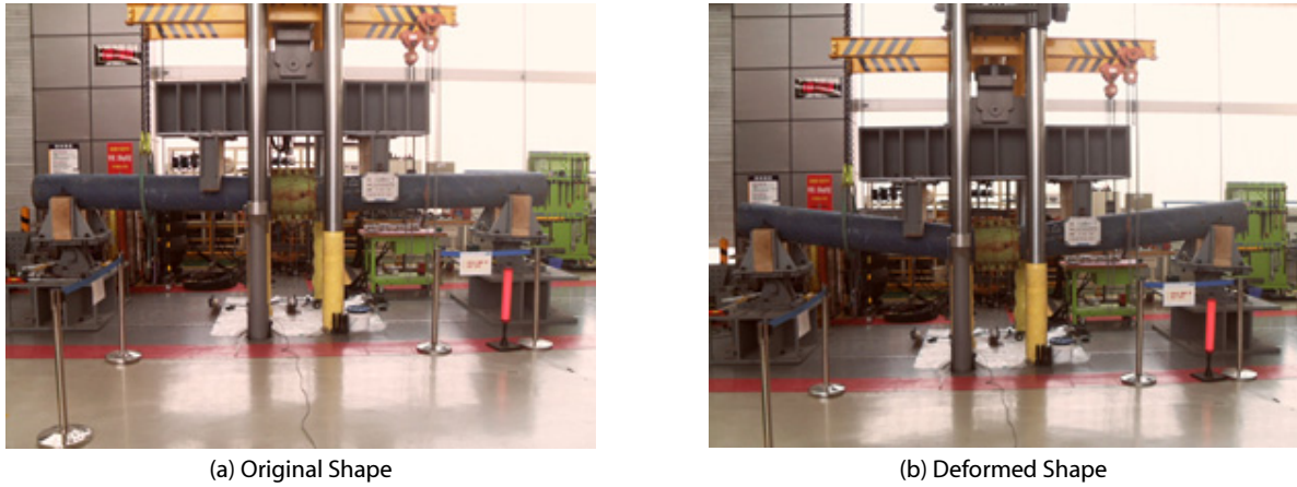
Fig. 2. Bending Experiments of Steel Pipes
