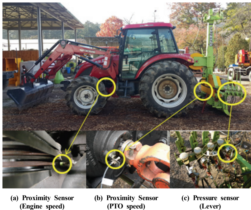
Figure 4. Sensor location of pressure and rotational speed for traction analysis.
