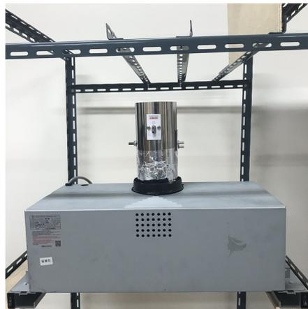
Fig. 5 Airflow measurement of kitchen hood using Debimo Blade
