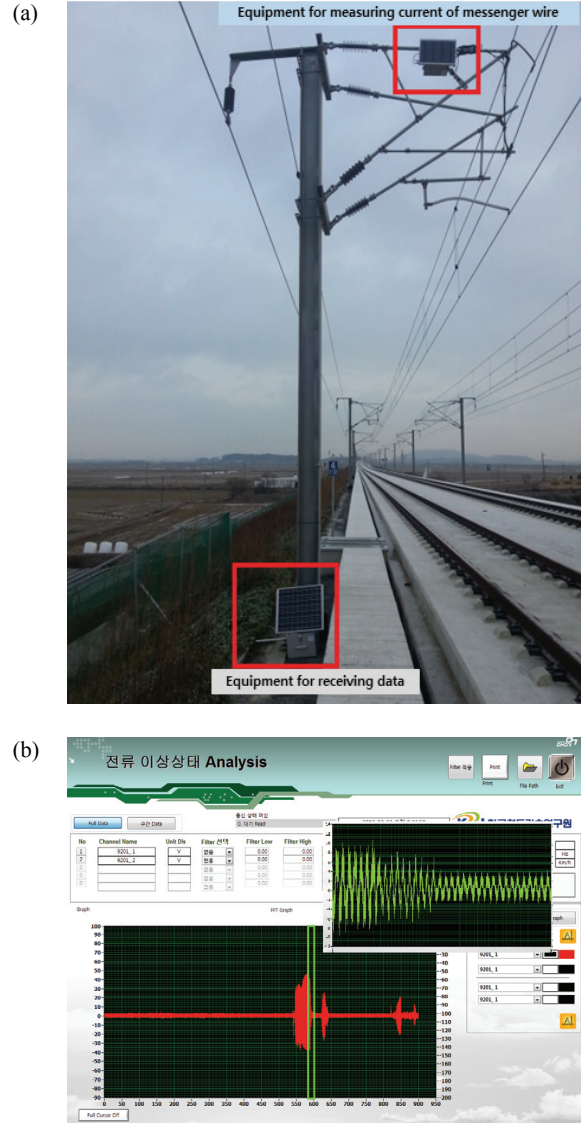
Fig. 1. Picture of current monitoring system, (a) installation of current monitoring system on OCL (overhead contact line) in Honam high-speed line and (b) program for analysis of current.
