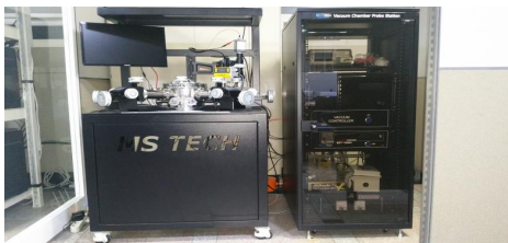
Fig. 12. Image of probe station (Voltage: -200V \sim 200V , Current level: < 10^{12} A) equipment.
