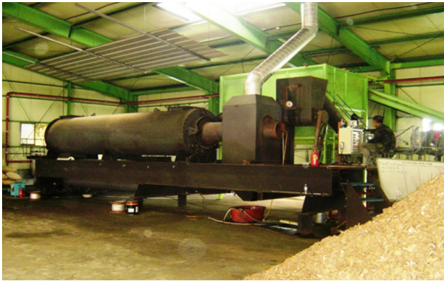
Fig. 3. Rotary kiln for the carbonization (Courtesy of Seyoung Co. Ltd.).
