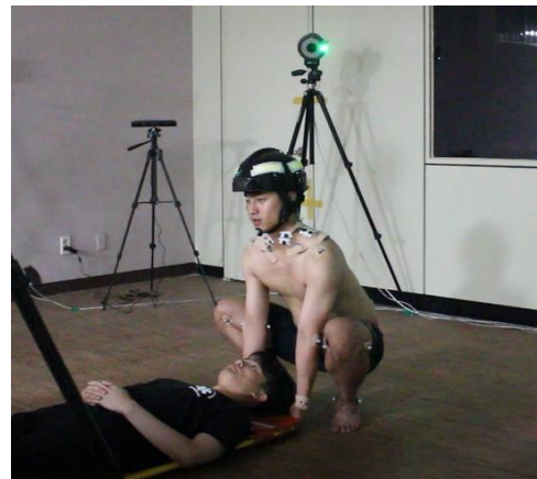
Fig. 2. Muscle activity mesure and position of upper body when lowering the stretcher
