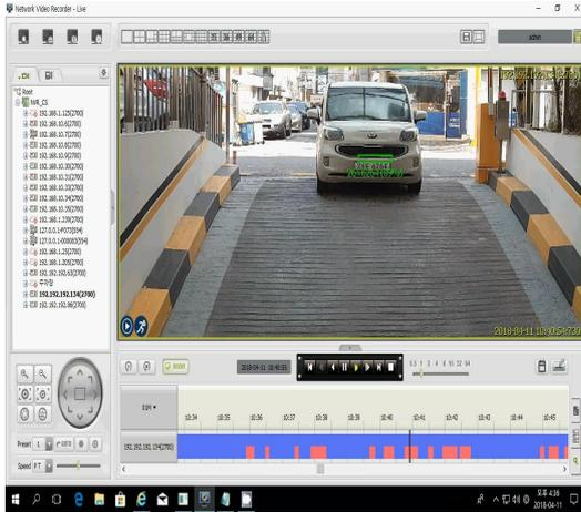
Fig. 9. Extraction and recognition for entering vehicle's license plate
