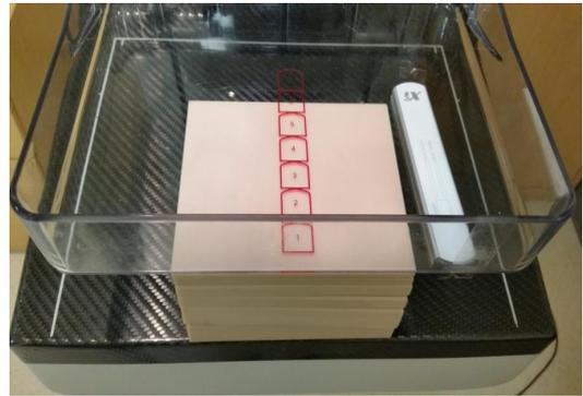
Fig. 3. Position of phantom and dosimeter for measurement of AGD
