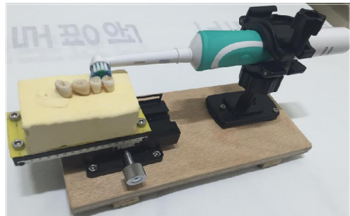
Fig. 3. Handmade Electronic Toothbrush Equipment
