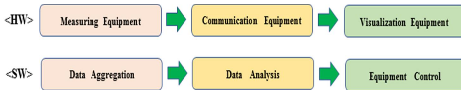
Figure 1. BEMS Technology Overview Diagram
