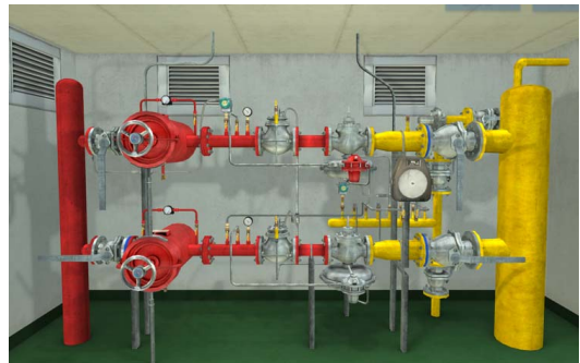
Fig. 1. Virtual model of city gas governor
