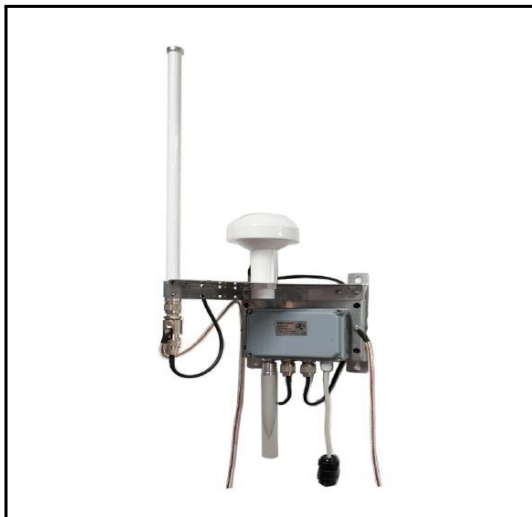
Fig. 5. LoRa to TCP/IP Gateway.
