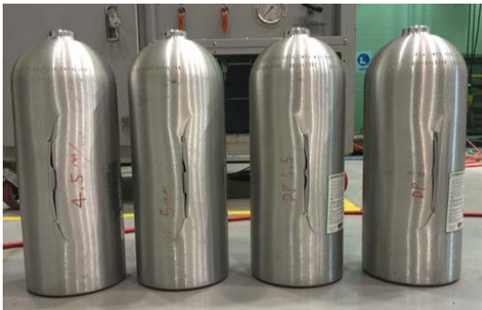
Fig. 4. After Rupture of cylinder specimen
