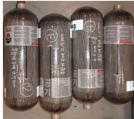
c. Composite cylinder specimen
