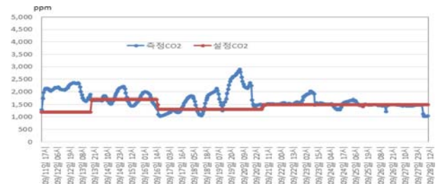
Fig 5. Setting and measuring CO 2 concentration during culture period of farm A.
