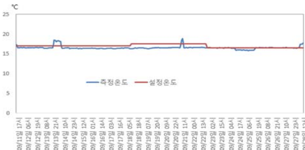
Fig 3. Setting and measuring temperature during culture period of farm A.
