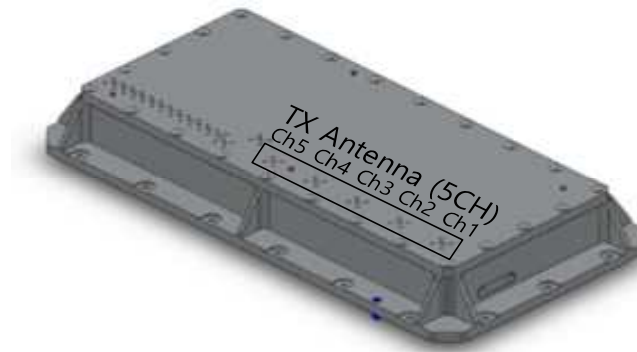
Figure 7. Transmitter configuration of W-band module
