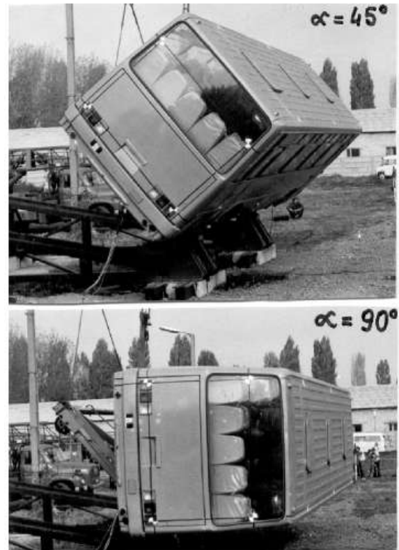
Fig. 2 Bus rollover test (7)
