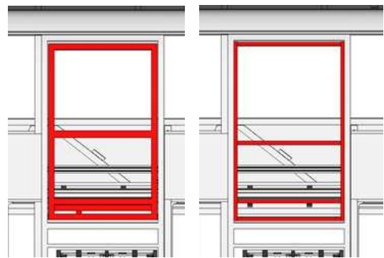
Fig. 5 Two types of the door models for wheelchair buses
