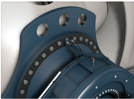
Fig. 1. Example of a previously developed rotating shaft bearing temperature sensor
