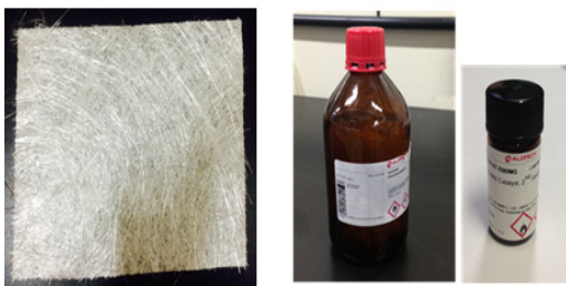
Fig. 1. Glass strand mat (left), DCPD resin and Grubbs 2nd catalyst (right)
