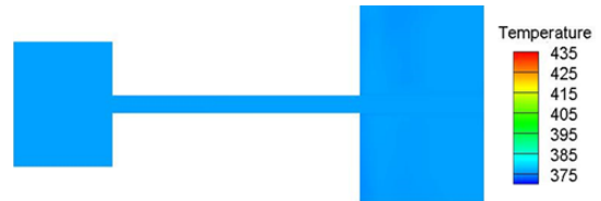
Fig. 7. Temperature distribution for inlet temperature of 103°C
