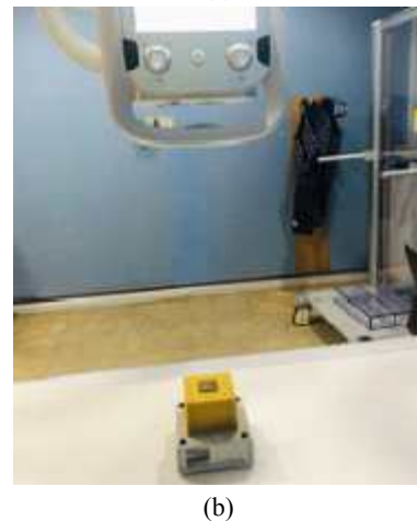
Fig. 6. Measuring arrangement for radiation shielding sheet.
