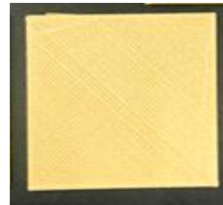
(a) radiation shielding sheet
