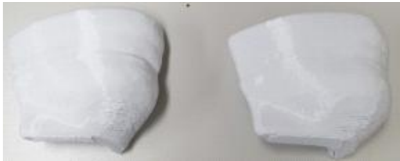
A : Bolus filled inside: PLA 5mm, 10mm
