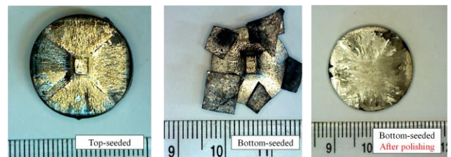
Fig. 5. Digital pictures of the melt-processed YBCO bulk specimen prepared (a) by a TSMG method, (b) and (c) by a BSMG method. (c) is the picture after polishing of (b).
