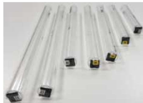
Fig. 4. Nanodot dosimeter attached on the acrylic tubes.
