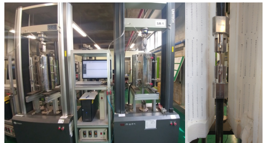
Fig. 2 Creep test machine and installed specimen
