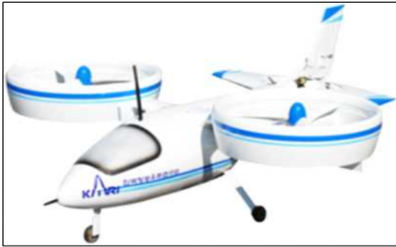
Fig. 2 The Ducted Fan UAV Configuration
