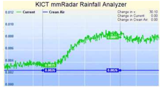
Fig. 12. The rainfall intensity estimated by W-band FMCW radar at the time of changing from weak to strong rainfall.
