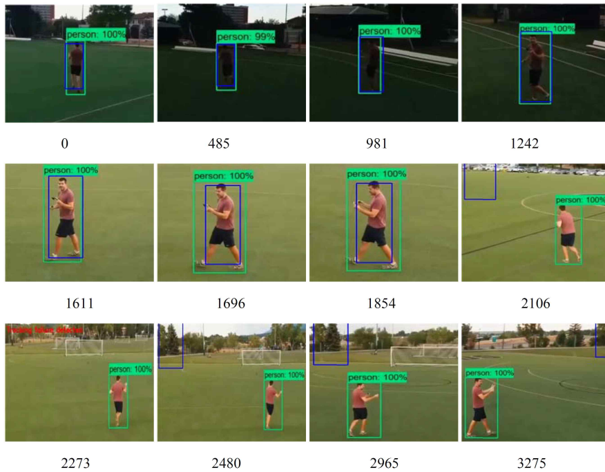
Fig. 15. Qualitative results of conventional (CSR-DCF, blue) and proposed (FRCNN_CSRT, green) trackers (0, 485, 981, ... - frames) .
