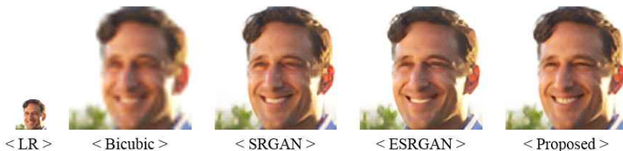
Fig. 2. SR results for various SR algorithms. The input image is 04723 from [10]. Scale factor is x4 and the size of LR image is 36×36.
