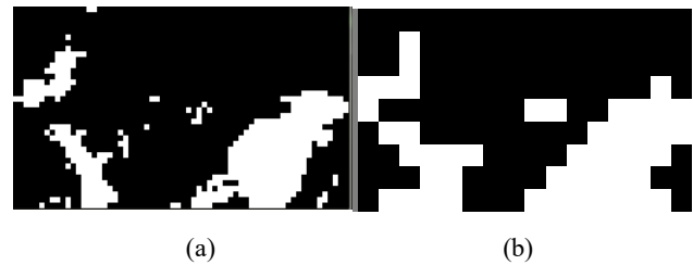
Fig. 3. Final detected ROI after removing small areas in a difference image; (a) a difference image filtered by the proposed method, (b) a final image of ROI detection after a small area is removed. (A pixel corresponds to a 40x40 block in an original image.)
