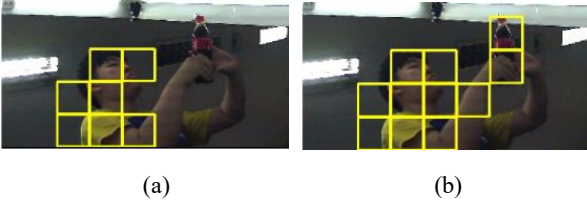
Fig. 5. Accuracy improvement by using an adaptive threshold; (a) ROI obtained by using a fixed threshold, (b) ROI obtained by using a spatiotemporally adaptive threshold.
