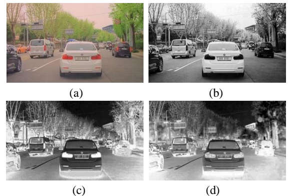
Fig. 2. Results after applying different weights for each channel: (a) input image, (b) Y channel, (c) U channel, and (d) V channel.
