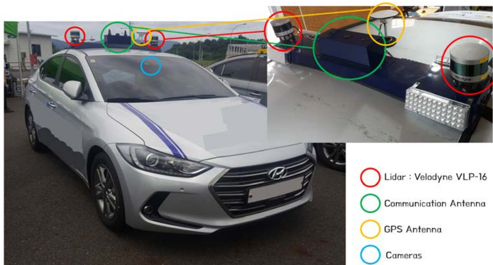
Fig. 9. An example of the test platform for a self-driving car
