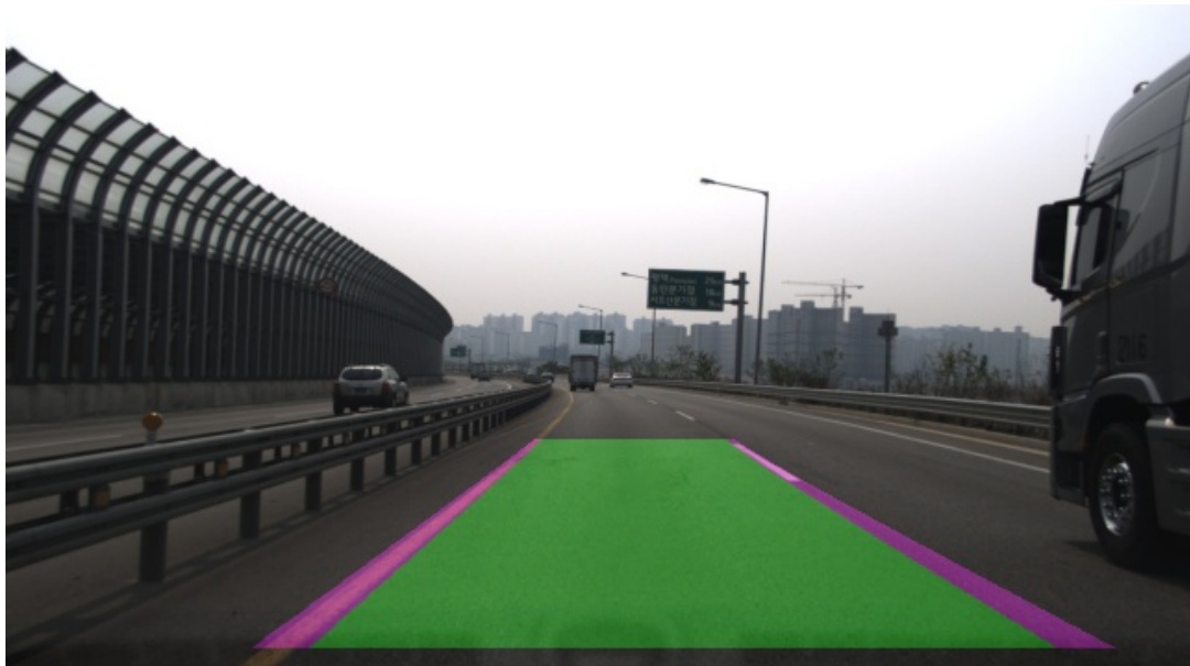
Fig. 2. Example of a lane detection result based on three image-processing methods: Sobel, perspective transform, and sliding window search.
