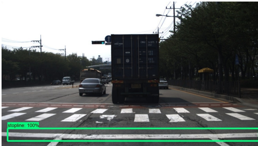
Fig. 3. Example of stop line detections using faster R-CNN inception V2
