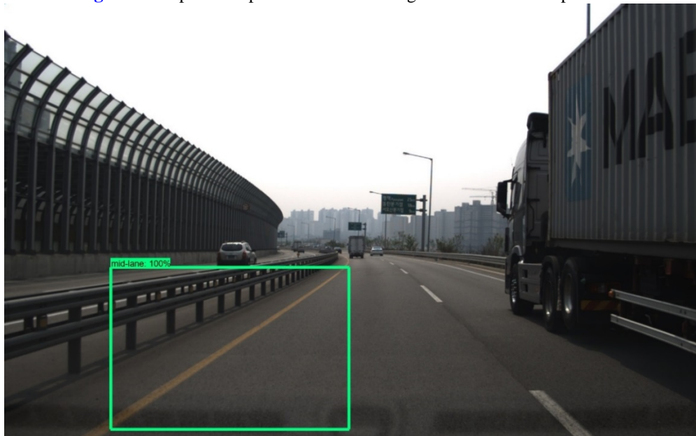
Fig. 4. Example of center line detections using faster R-CNN Inception V2
